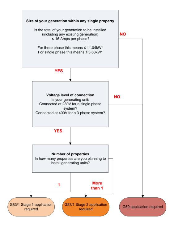
There are three types of distributed generation connection. This flowchart will help you to understand which type of connection application you need to make
