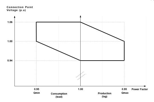
Figure 13.8 Reactive Power capability requirements (Power Park Modules operating at Registered Capacity)
