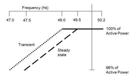
Figure 13.1 Change in Active Power with falling frequency
