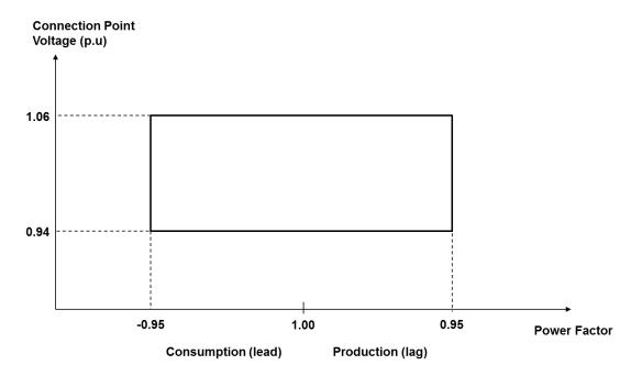
Figure 13.6 Reactive Power capability requirements (Synchronous Power Generating Modules operating at Registered Capacity)
