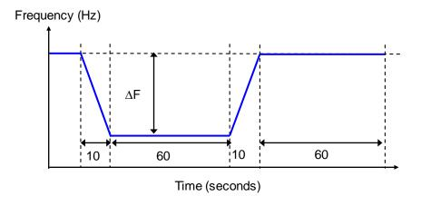
Figure C.7.3 LFSM-U step response simulation
