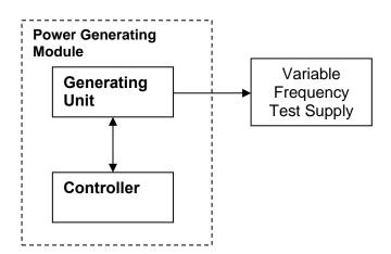
Figure A.7.6. set up – over / under frequency
