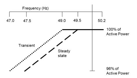
Figure 11.1 Change in Active Power with falling frequency
