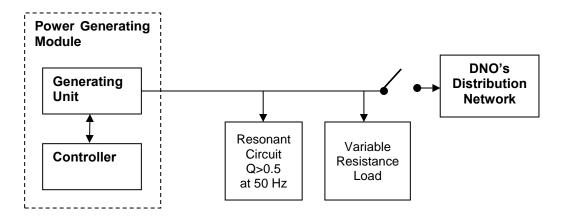
Figure A.7.7 set up - loss of mains
