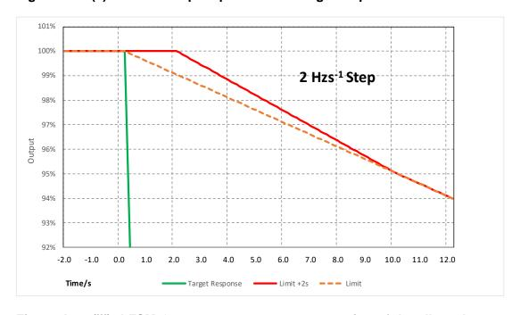
Figure A.7.8(iii): LFSM-O step response test – expansion of the allowed 2 s response delay (frequency increase)
