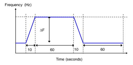
Figure B.4.1 – LFSM-O frequency step response simulation
