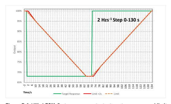
Figure B.6.1(ii): LFSM-O step response test - target response and limits
