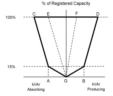
Figure 12.4 Generator Performance Chart at Connection Point - Power Generating Facilities
