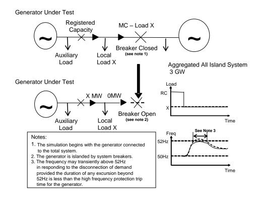
Figure C.7.1 - Diagram of Load Rejection Study
