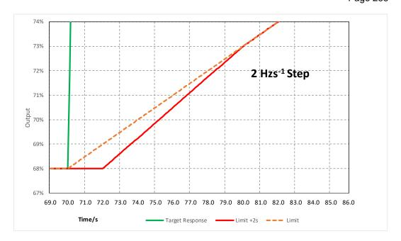
Figure B.5.1(vi): LFSM-O step response test – expansion of the allowed 2s delay (frequency decrease)
