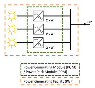
Figure 4.2 (a) 3 x 2 kW Inverter connected Generating Units
