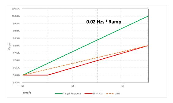
Figure B.5.2(iv): LFSM-O ramp response test – expansion (frequency decrease)
