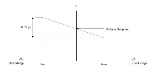
Figure 12.5 Voltage control with Slope
