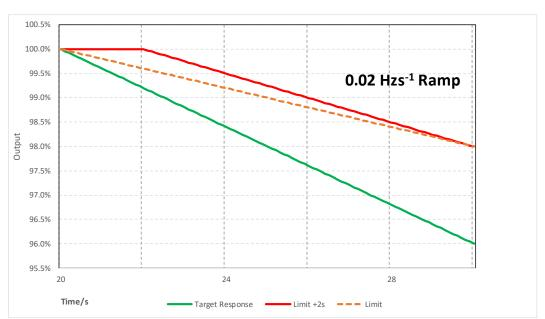
Figure A.7.9(ii): LFSM-O - target response and limits
