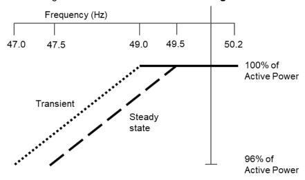
Figure 12.1 Change in Active Power with falling frequency
