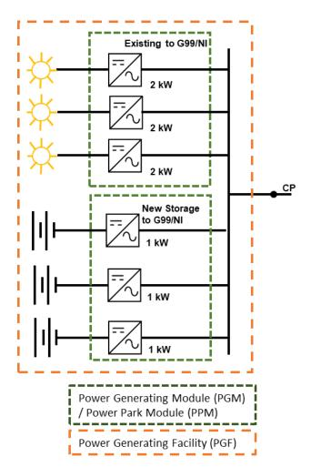
Figure 6.7. Example: Existing 6 kW Type A Power Park Module to EREC G99/NI plus later addition of 3 x 1 kW Electricity Storage devices with own Inverters
