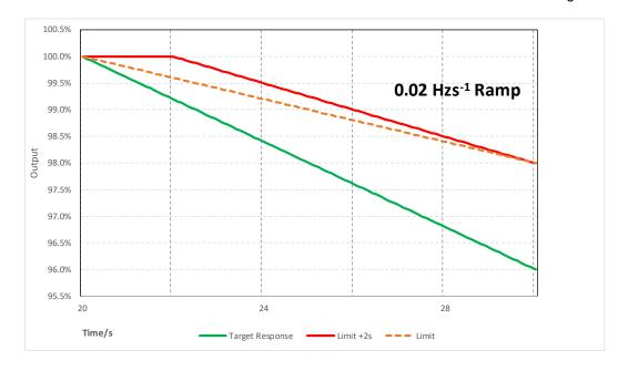
Figure B.5.2(iii): LFSM-O ramp response test – expansion (frequency increase)
