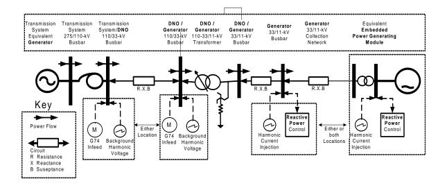
Figure 6.8 Example equivalent Total System representation
