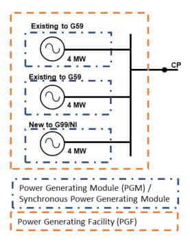
Figure 6.3. Example: Existing:  $2 \times 4$  MW Type B Synchronous Power Generating Modules with new unit =  $3 \times 4$  MW Type B Synchronous Power Generating Modules
