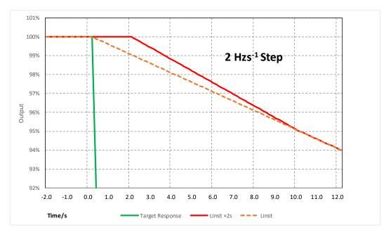
Figure B.5.1(iii): LFSM-O step response test – expansion of the allowed 2s delay (frequency increase)
