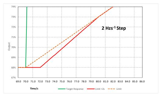
Figure B.6.1(iv): LFSM-O step response test – expansion of the allowed 2s response delay (frequency decrease)
