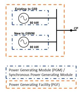
Figure 6.1. Example: 1 x 80 kW Synchronous Power Generating Module to EREC G59 plus 1 x 80 kW Type A Synchronous Power Generating Module to EREC G99/NI
