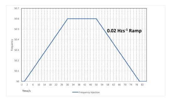
Figure B.5.2(i): LFSM-O ramp response test – frequency injection
