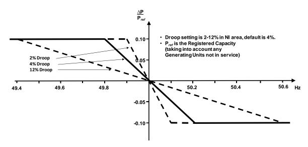
Figure 13.2 – Frequency Sensitive Mode capability of Power Generating Modules and Power Park Modules
