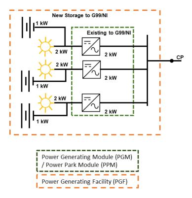
Figure 6.6. Example: Existing 6 kW Type A Power Park Module to EREC G99/NI plus later addition of  $3 \times 1$  kW Electricity Storage devices (Compliance remains the same)
