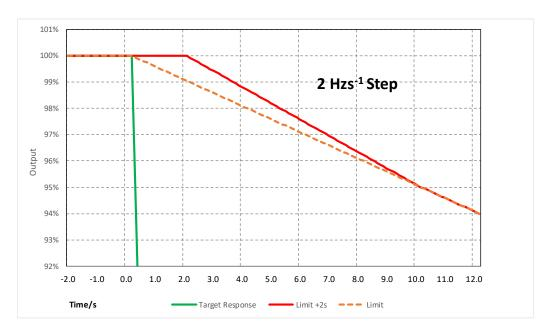
Figure B.6.1(iii): LFSM-O step response test – expansion of the allowed 2s response delay (frequency increase)
