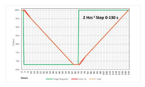
Figure B.5.1(ii): LFSM-O step response test – target response and limits
