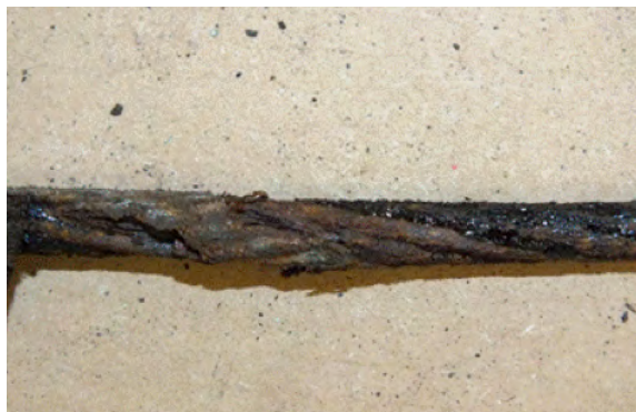
Corrosion of 110kV line between Ballylumford and Castlereagh.
