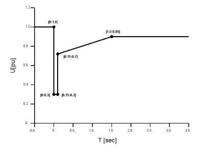
Fault Ride Through capability for Power Stations < 5 MW
