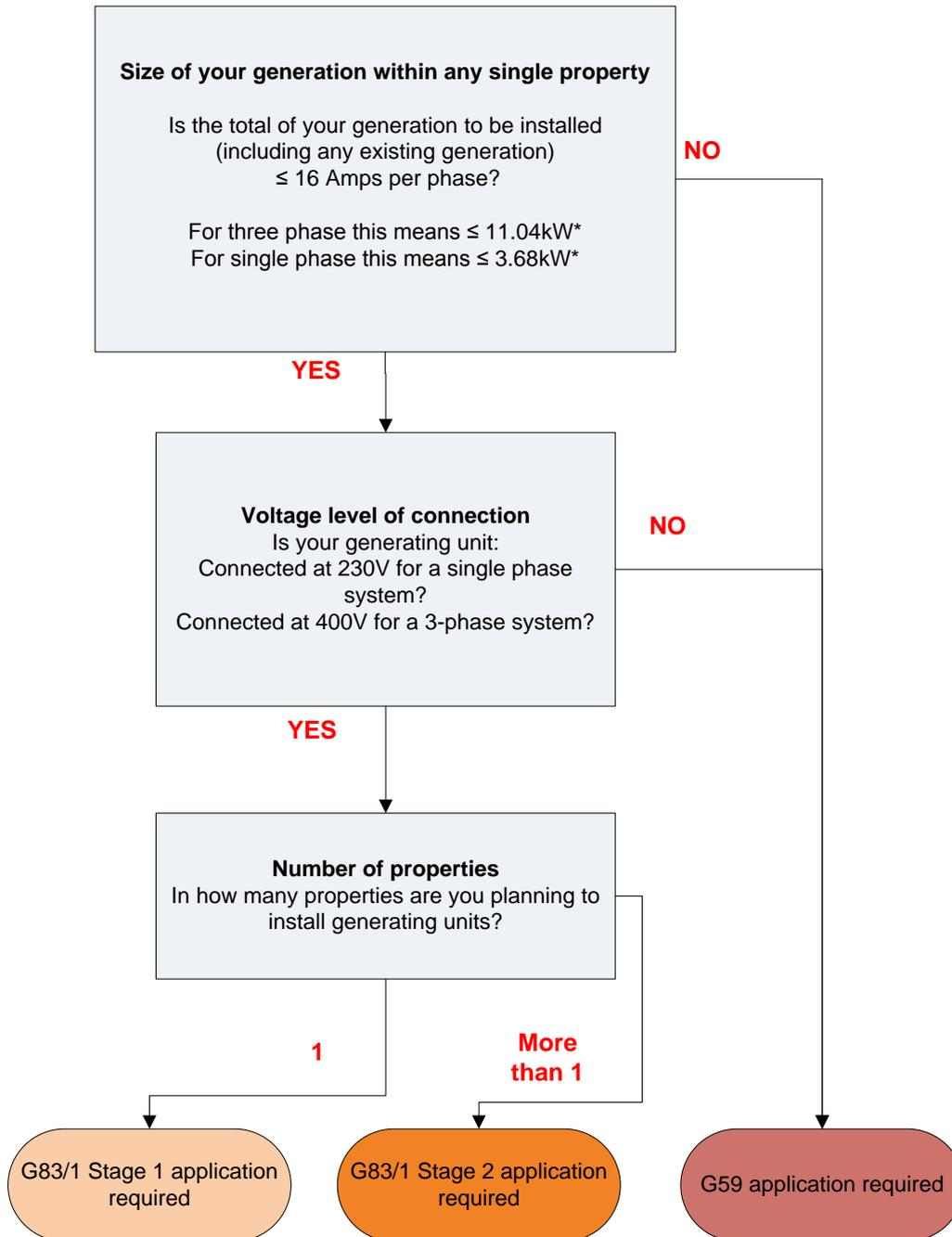
There are three types of distributed generation connection. This flowchart will help you to understand which type of connection application you need to make
